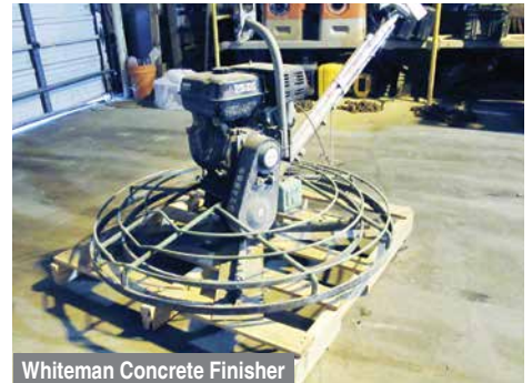
Whiteman Concrete Finisher
